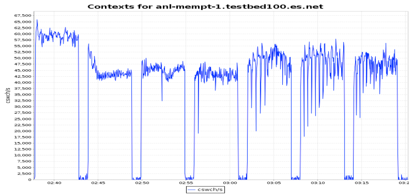
Figure 12: ANI testbed 100Gbps (10x10NICs, three hosts): Context switches vs the number of concurrent transfers [1, 2, 4, 8, 16, 32 64 concurrent jobs - 5min intervals], TCP buffer size is 50M
