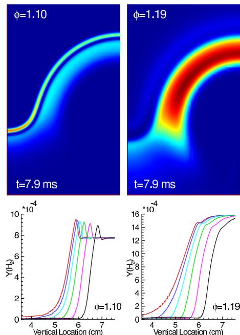
**Fig. 4** -  $H_2$  diffusion flux  $|\rho D_{H_2} \nabla Y_{H_2}|$  for  $\phi = 1.10, 1.19$  at 7.9 ms. Also,  $H_2$  mass fraction along vortex centerline (right domain boundary) at selected times in the range  $0 \leq t \leq 7.9$  ms. The broader  $Y_{H_2}$  profile for  $\phi = 1.19$  is scoured out of the region in front of the flame by the approaching vortex, enhancing diffusive transport. The narrow  $Y_{H_2}$  profile for the  $\phi = 1.10$  case is not similarly affected.
