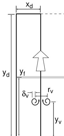
**Fig. 1** - Schematic of the premixed methane flame-vortex problem. The shaded line represents the position of the flame, and the swirl lines represent the initial vortex. We impose symmetry along the sides of the  $0.8 \times 4.0$  cm domain to avoid modeling the dotted region.
