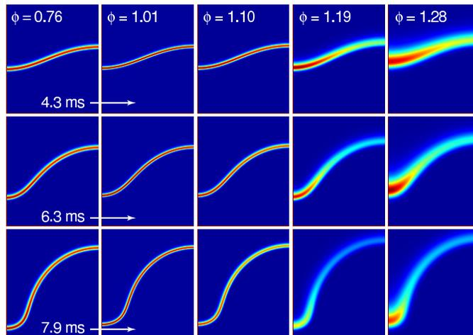
**Fig. 2** - CH mole fraction. In each column, the three frames correspond approximately to 4.3, 6.3 and 7.9 ms simulation time from the initial conditions (see Fig 1). The color scale in each column is normalized to peak values of  $X_{\text{CH}} = 0.23, 7.76, 10.8, 3.66, 0.30 \times 10^{-7}$ , respectively. The frames represent  $8 \times 9.5$  mm subregions of the domain near the flame surface.
