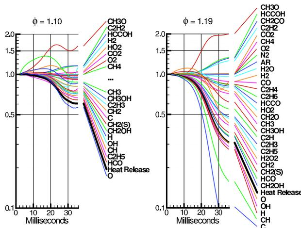
**Fig. 3** - Time history of the peak values of molar concentration, normalized to their respective values at  $t = 2$  ms. Normalization is made at this later time to avoid initial transients as the PREMIX solution adjusts to the AMR grid. Note these data are taken from simulations on very large  $1.2 \times 5.6$  cm domains to avoid edge effects at later times in the flame vortex interaction.
