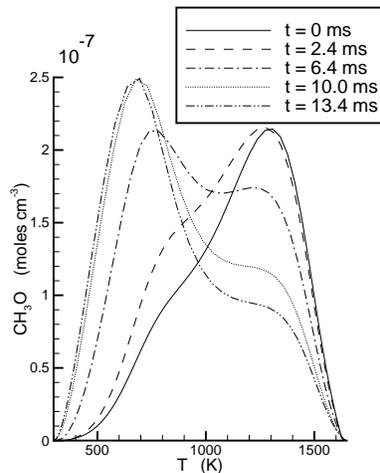
**Fig. 5** -  $\text{CH}_3\text{O}$  profiles along the vortex centerline for  $\phi = 1.19$ . During the flame-vortex interaction, there is a marked enhancement of  $\text{CH}_3\text{O}$  concentration in low temperature regions.
