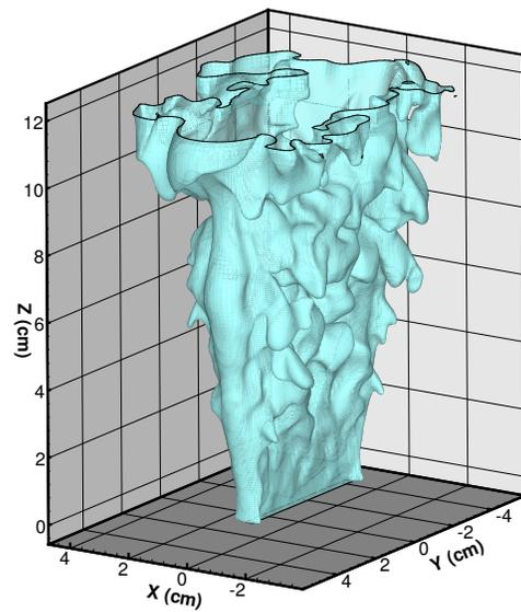
Figure 4: The computed  $c = 0.5$  flame surface.
