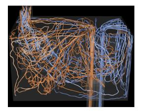
Figure 5: A thermal hydraulics simulation from the NEK5000 code. The streamlines show the behavior of warm and cool air inlets (orange and blue respectively) and representative behavior for how long particles remain in the assembly before exiting through the outlet (top left).
