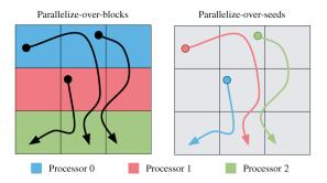
Fig. 1. Immediate parallelization approaches for distributed streamline integration. *Parallelize-over-blocks* (left) relies on a fixed assignment of data blocks to processors and passes streamlines between processor as they advance into new blocks. *Parallelize-over-seeds* (right) distributed streamlines evenly among processors and data blocks are loaded on demand when required to integrate a streamline.
