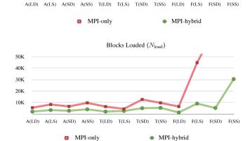
Fig. 5. A comparison of performance for hybrid and nonhybrid variants of the *parallelize-over-seeds* algorithm, in terms of the metrics from Section 4.4. The hybrid version is faster in all cases because fewer blocks are loaded, allowing for an increased integration ratio. See Section 5.1 for a detailed discussion.
