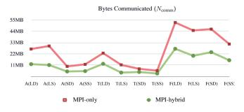
Fig. 6. Performance of hybrid versus nonhybrid variants of the *parallelize-over-blocks* algorithm as measured according to Section 4.4. The hybrid version has strongly decreased runtime for the same test because reduced communication enables a higher integration ratio is higher. See Section 5.2 for a detailed discussion.
