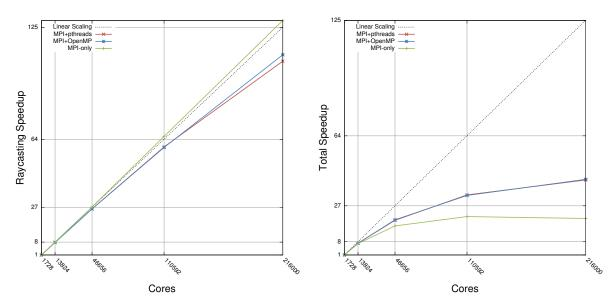
Figure 2: The speedups (referenced to 1,728 cores) for both the raycasting phase and the total render time (raycasting and compositing).
