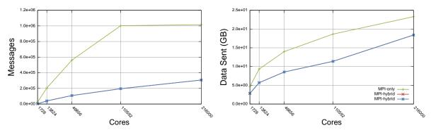
Figure 3: The number of messages and total data sent during the compositing fragment exchange.
