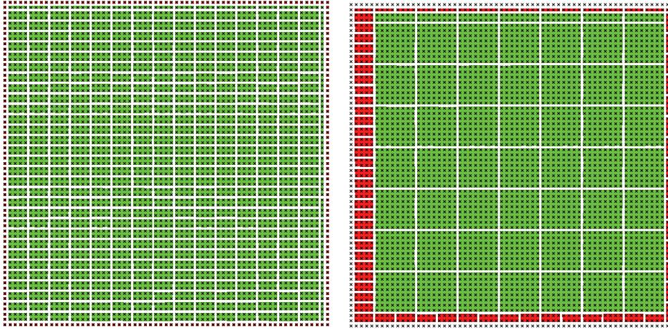
FIG. 5. Aggregation for the model Poisson problem on the unit square with  $h = 1/64$ : result of the multiple pairwise aggregation algorithm with three passes at level 1 (left) and level 2 (right).
