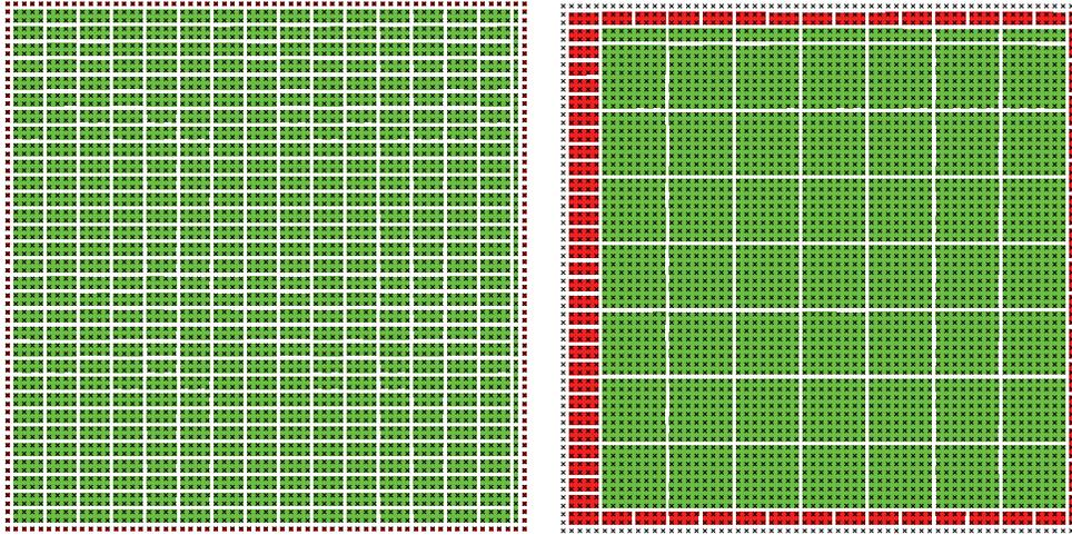
FIG. 6. Aggregation for the model Poisson problem on the  $1 \times (1 + h)$  rectangle with  $h = 1/64$ : result of the multiple pairwise aggregation algorithm with three passes at level 1 (left) and level 2 (right).
