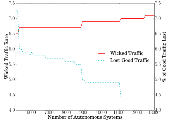
Figure 9: Change wicked traffic and loss of legitimate traffic over time as the network grows from 5 000 to 13 000 ASes. The wicked traffic rate is the percentage of all traffic that is wicked.
