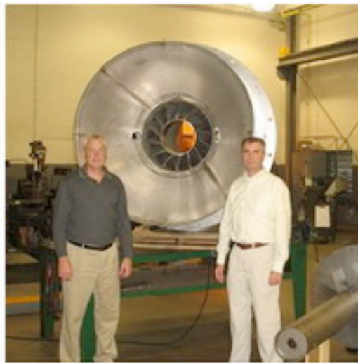
28" burner (44 MW, 150 MBtu/hr)
