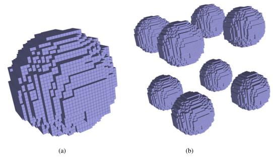
**Figure 1.** (a) Grids at the finest AMR level used in the hyperbolic gas dynamics benchmark – these grids cover the shock front of a spherical explosion in 3D. (b) Replicated grids at the finest AMR level used in the weak scaling performance study of the hyperbolic gas dynamics benchmark.
