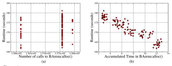
**Figure 4.** Scatterplot (a) shows no correlation between the run time variation and the number of memory allocations performed. Scatterplot (b) shows a clear anti-correlation between the time spent in the memory allocation routines and the runtime variation – meaning that processors that showed the slowest runtime spent the least time in performing memory allocation, despite a balanced workload.
