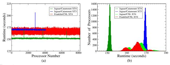
**Figure 2.** (a) Runtime of each MPI process rank on *Jaguar*/Catamount and *Franklin*/CNL. The spikes in the *Jaguar*/Catamount runtimes were attributed to ECC memory correction overhead on nodes experiencing high memory error rates. (b) Histogram of runtime variability for the AMR hyperbolic gas dynamics runs on the evaluated systems.
