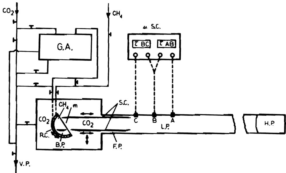
Figure 2. Layout of apparatus. G.A. thermal conductivity gas analyser;  $\mu$  S.C. micro-second counter; S.C. shock cutter; L.P. low pressure driver section,  $CO_2$ ; H.P. high pressure driving section with air as driver gas; V.P. vacuum pump; B.P. back plate; F.P. front plate.
