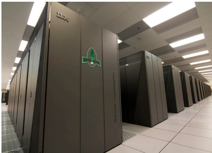
Sequoia, an IBM BlueGene/Q system, was the first supercomputer with more than 1 million cores. It comprises 1,572,864 cores and 1.6 petabytes of memory.
