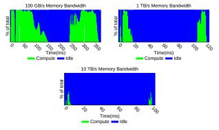
Fig. 10: Percentage of time the V-cycle spends computing versus waiting for communication to complete over time for three memory bandwidth values.
