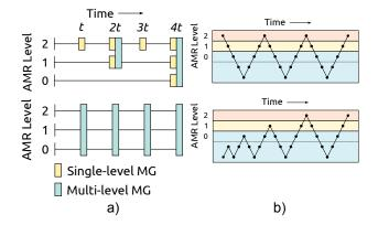
Fig. 3: a) A comparison between AMR simulation with and without subcycling; b) A comparison between multigrid V-cycles and F-cycles
