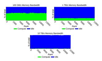
Fig. 9: Percentage of time each rank spends computing versus waiting for communication to complete for three memory bandwidth values.
