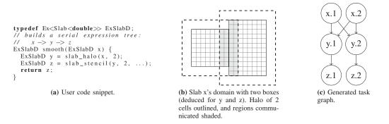
Fig. 2: An example of how ProgrAMR generates the task graph given an expression tree and initial mesh configuration.
