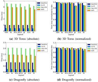
Fig. 4: A comparison of box layout algorithms in the larger, balanced case for different network latency configurations. Both absolute time and normalized time vs. random are shown.
