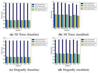
Fig. 7: A comparison of asynchronous execution models in the larger, balanced case for different box layout algorithms. Both baseline and latency-modified configurations are shown.
