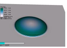
Impact of automatic timestep control: dome problem after 1 year of simulation time. (left) Original BISICLES integrator – note ridges near center which indicate numerical instability. (center) Using SUNDIALS automatic timestep control – note smoothness of upper surface. (right) Requested timesteps (green) vs. actual limited timestep (blue), and actual timestep with a tighter solution error tolerance (which results in more-conservative timesteps).
