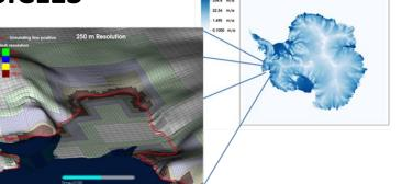
BISICLES-computed Antarctic ice velocity field. Inset shows adaptive meshing near the Pine Island Glacier grounding line.
