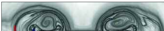
Figure 3. Pathlines are seeded according to FTLE strength, FTLE ridge lines, or via a user-guided probability density function (PDF). The top image shows visualization of primary (red) and secondary (blue) separation structures; pathlines are seeded according to the PDF shown in the lower image, which shows the planar FTLE visualization on a section plane perpendicular to the main flow direction. Darker regions correspond to regions of high FTLE. Colored regions indicate PDFs used to see the pathlines in the upper right image.
