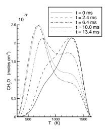
Fig. 5 - CH<sub>3</sub>O profiles along the vortex centerline for  $\phi = 1.19$ . During the flame-vortex interaction, there is a marked enhancement of CH<sub>3</sub>O concentration in low temperature regions.
