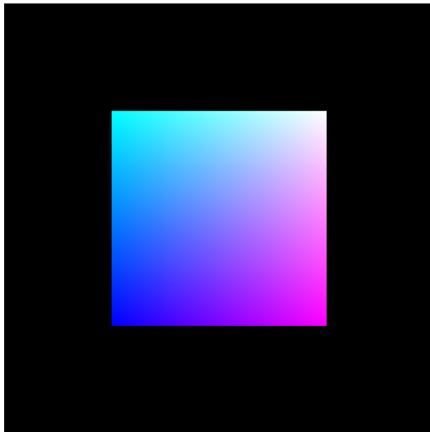
Figure 1: The wesBench application generates triangles that fill approximately 1/4 of the screen with triangles, and then rotates those triangles about the center of the screen over the course of the benchmark. This image shows the unlit disjoint triangles that are the basis for the geometry/rasterization crossover experiment.
