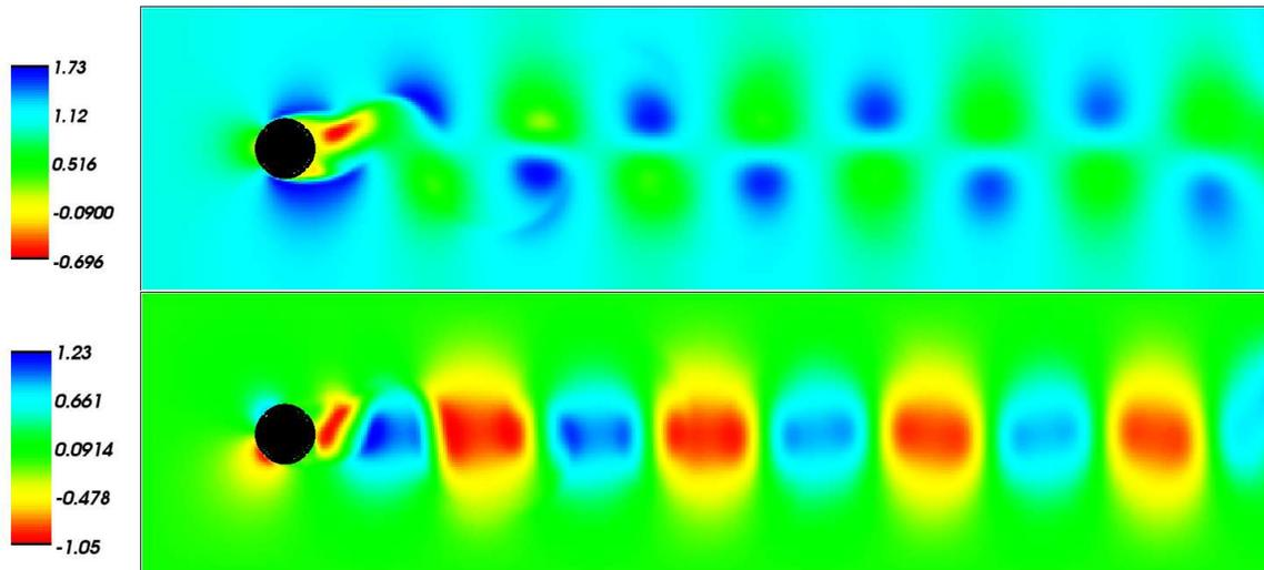
Fig. 11. Embedded boundary calculation of two-dimensional flow over a circular cylinder. The upper figure is the axial velocity, the lower is the transverse velocity. The grid resolution is  $512 \times 128$ . The Reynolds number based upon the diameter is 500. The velocity at inflow is 1.0. There have been 12000 time steps taken and  $t=25.56$ .
