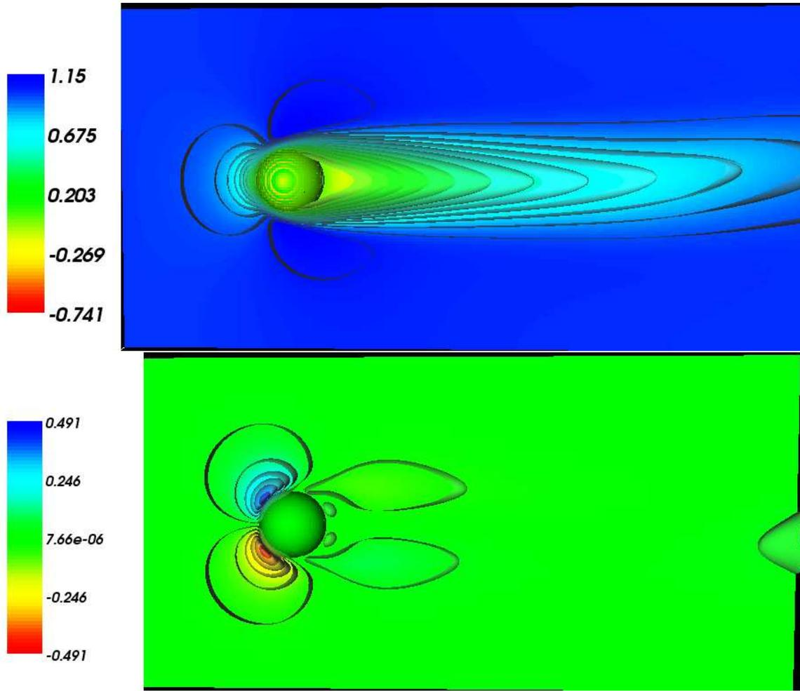
Fig. 12. Embedded boundary calculation of three-dimensional flow over a sphere. The upper figure is the axial velocity, the lower one the transverse velocity. The grid resolution is  $256 \times 128 \times 128$ . The Reynolds number based upon the diameter is 100. The velocity at inflow is 1.0. There have been 600 time steps taken and  $t=1.96$ .
