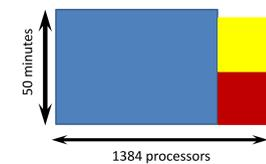
Illustration of POPSICLES work distribution during a single coupling interval. Blue: POP2x, Red: BISICLES, Yellow: POPSICLES setup for next interval
