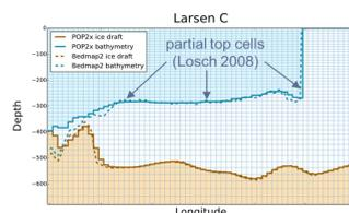
In POP, partial bottom cells discretize bathymetry. POP2x extends this approach to include partial top cells at upper ice-shelf/ocean boundaries, allowing computation of circulation in ice-shelf cavities.
