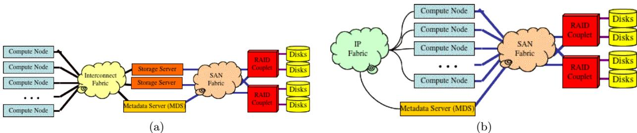
**Figure 1: The general architecture of cluster filesystem we have studied, including Lustre, PVFS2, and GPFS, follow the abstract pattern shown in (a); the CXFS configuration is more similar to a SAN, shown in (b).**
